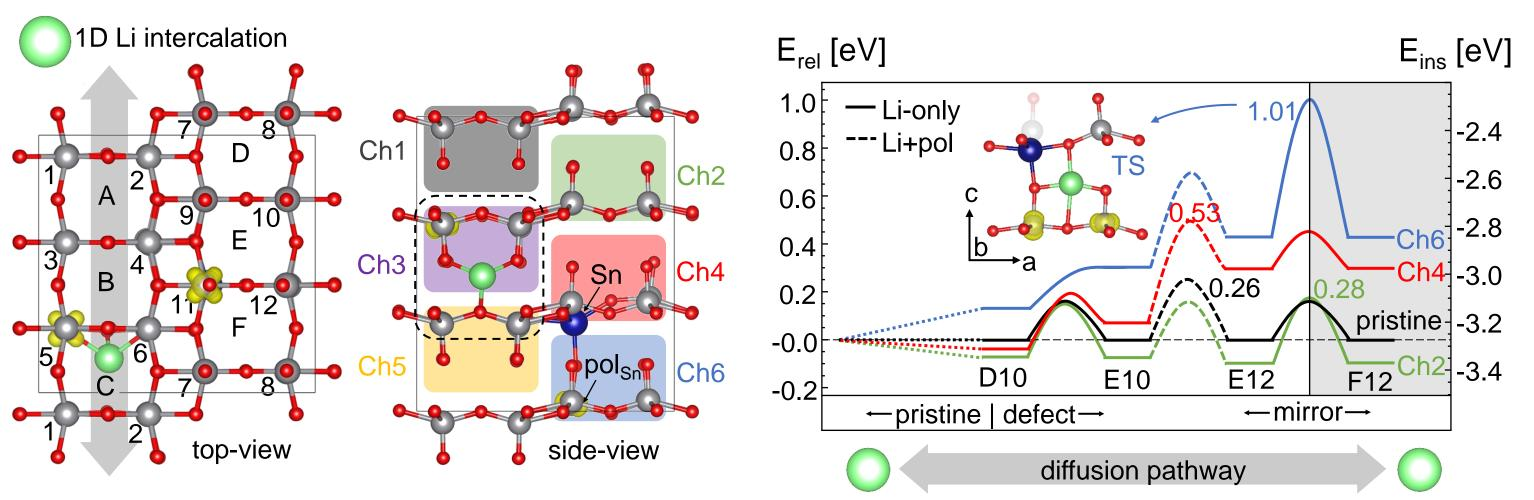
The Sn defect center could slow down Li-coupled polaron diffusion with effective barrier of 1.01 eV
