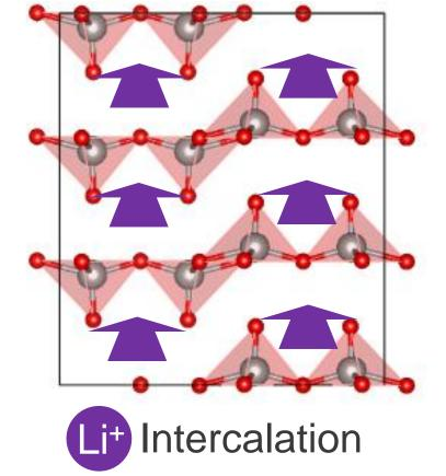
$\Box$  Layered structures of V<sub>2</sub>O<sub>5</sub>  $\rightarrow$  accommodate Li<sup>+</sup> □ It can be used as cathode materials.
